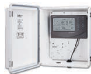
Complete System Shelter with Vantage Pro2 console.
