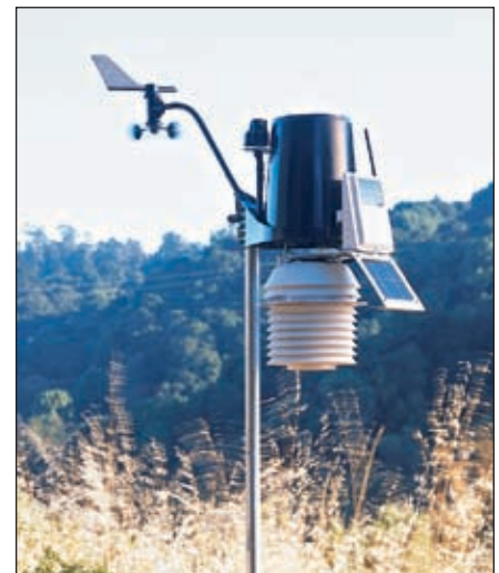
6328 with 24-Hour Fan-Aspirated Radiation Shield
